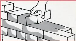
Trowel or dip contact surfaces of brick, slide into place.
