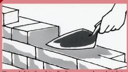
Trowel thin "cushion" of mortar where brick is to be laid.
