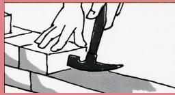
Tap brick firmly with hammer against side as shown.
