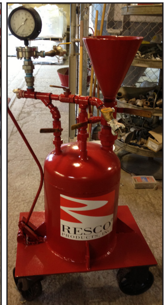
PRESSURIZED JAMB SPRAY VESSEL
